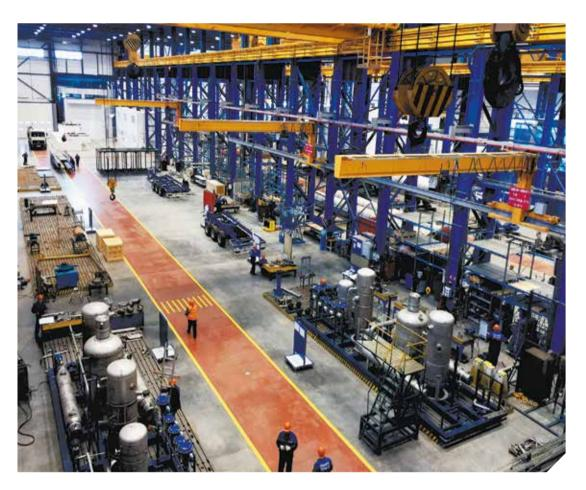
he production capacities of Cryogenmash allow for the manufacturing of cryogenic, chemical and petrochemical products with the following max dimensions: 40,000x5,500x4100 mm (LxWxH) and a weight of up to 80 tons for packaged modular equipment, and up to 4,500 mmi n diameter, up to 26,000 mm in length, and up to 60 tons in weight for vessels and apparatus.
