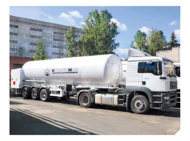
Cryogenmash manufactures transport tankers designed for liquid cryoproducts transportation, short-term storage and delivery to customers.
