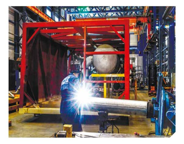
ur assembly and welding facilities are competent in flat rolled steer produce processing with a thickness of 1.0 to 40 mm. robotic plasma cutting of complex geometric profiles and robotic welding of steel and aluminum-alloy critical joints with a thickness of 4 to 40 mm.
