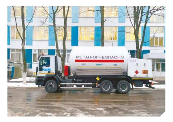
It is proposed to use road tankers and ISO tank containers to transport LNG from an LNG plant to other infrastructural facilities. In addition to transportation solutions, we offer a solution for mobile filling systems based on road tankers. A semi-trailer tanker consists of a tanker on chassis board, a pressurization evaporator and a valve rack where all control and monitoring instruments are installed.
