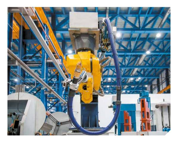
ryogenmash is the first in Russia to use Frobotics for welding of critical welded joints in the chemical and petrochemical industry. Robotic systems are used for plasma cutting and deseaming of steel and aluminum alloys, and also for welding of steel and aluminum alloys with shielding gas.
