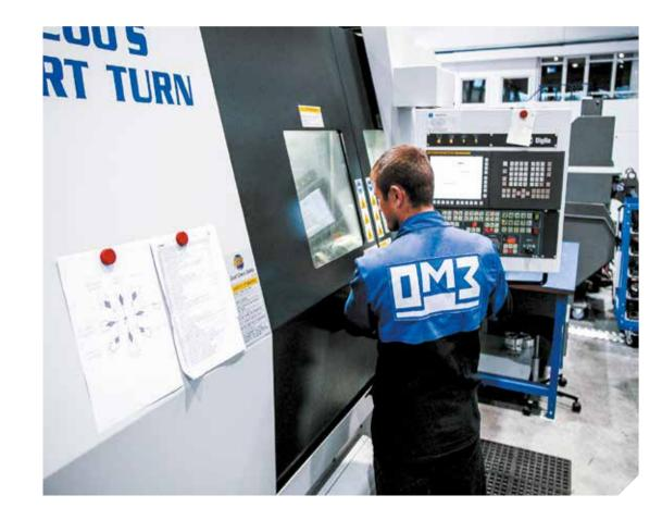
echanical production mainly includes machining centers that use the numerical program control technology and provide for precision mechanical processing (on the order up to 2 microns), with the maximum dimensions of up to 5,000 mm and the maximum workpiece weight of up to 12 tons. The equipment of world leaders of the European and Asian machine tool industry, such as HERMLE, BIGLIA, WELLE, is used.
