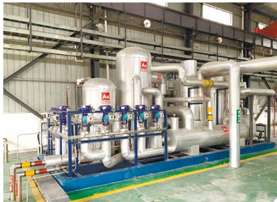
Cryogenmash's technology – the throttle-ejector cycle (0.3 to 4 tons of LNG per hour per line) – is optimal for the creation of mini LNG plants, as an alternative to gas pipelining, to supply natural gas to remote infrastructural facilities and gas engine vehicles within a radius 150 – 1,000 km:
