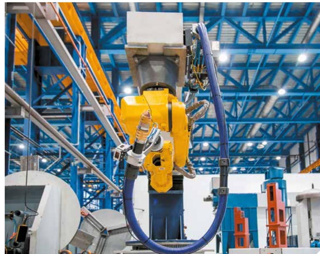
Cryogenmash is the first in Russia to use robotics for welding of critical welded joints in the chemical and petrochemical industry. Robotic systems are used for plasma cutting and deseaming of steel and aluminum alloys, and also for welding of steel and aluminum alloys with shielding gas.
