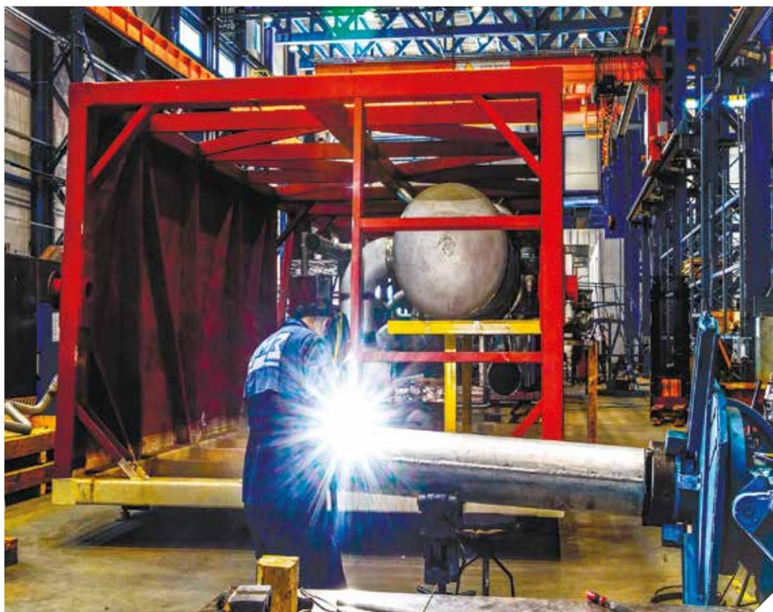
**O**ur assembly and welding facilities are competent in flat rolled steel products processing with a thickness of 1.0 to 40 mm. The production uses unique technologies, such as robotic plasma cutting of complex geometric profiles and robotic welding of steel and aluminum-alloy critical joints with a thickness of 4 to 40 mm.
