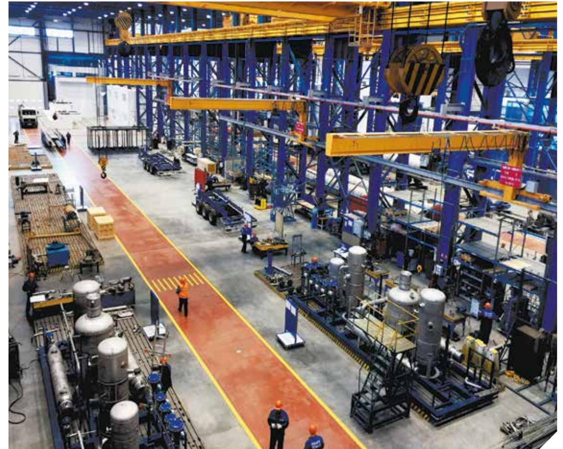
The production capacities of Cryogenmash allow for the manufacturing of cryogenic, chemical and petrochemical products with the following max dimensions: 40,000x5,500x4100 mm (LxWxH) and a weight of up to 80 tons for packaged modular equipment, and up to 4,500 mm in diameter, up to 26,000 mm in length, and up to 60 tons in weight for vessels and apparatus.
