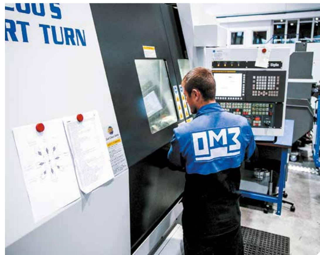
**M**echanical production mainly includes machining centers that use the numerical program control technology and provide for precision mechanical processing (on the order up to 2 microns), with the maximum dimensions of up to 5,000 mm and the maximum workpiece weight of up to 12 tons. The equipment of world leaders of the European and Asian machine tool industry, such as HERMLE, BIGLIA, WELLE, is used.
